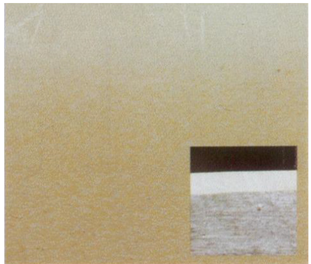
24. Yellowing Caused by Thick Gel Coat (Inset shows 55 mil thickness of white gel coat)
